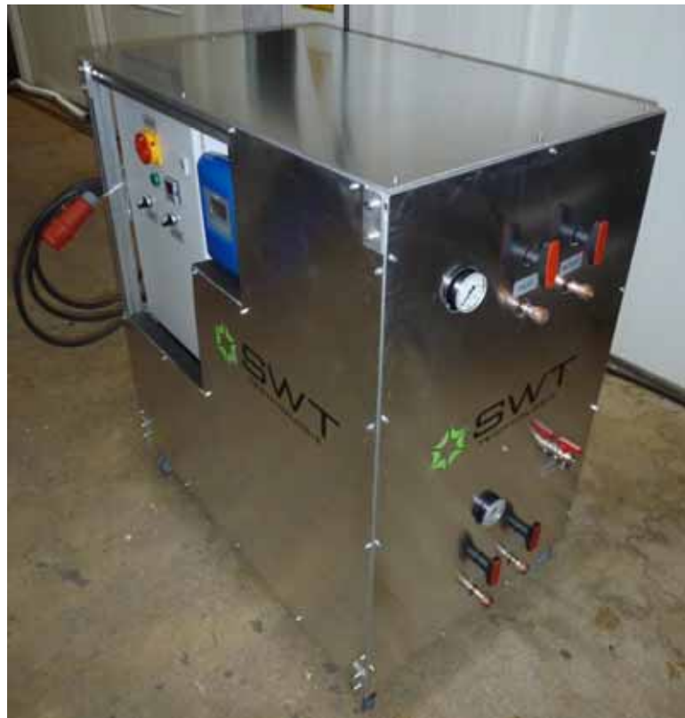
Figure 2: Module for testing the thermal performance of hot water stores acc. to EN 12977-3
