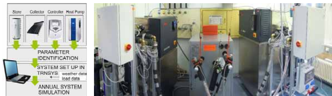
Fig. 1: Schematic procedure of the CTSS method extended to heat pump systems and picture of the laboratory test facility
