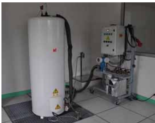
Figure 3 : Experimental set-up to evaluate the concept of PV DHWS
