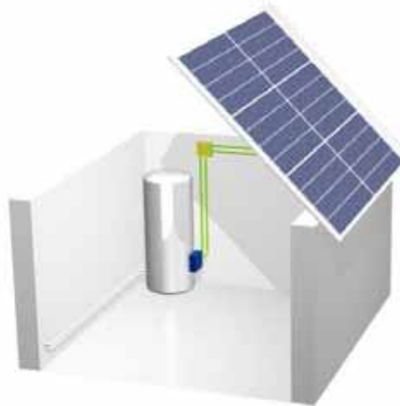
Figure 2 : Concept of a PV Domestic Hot Water System
