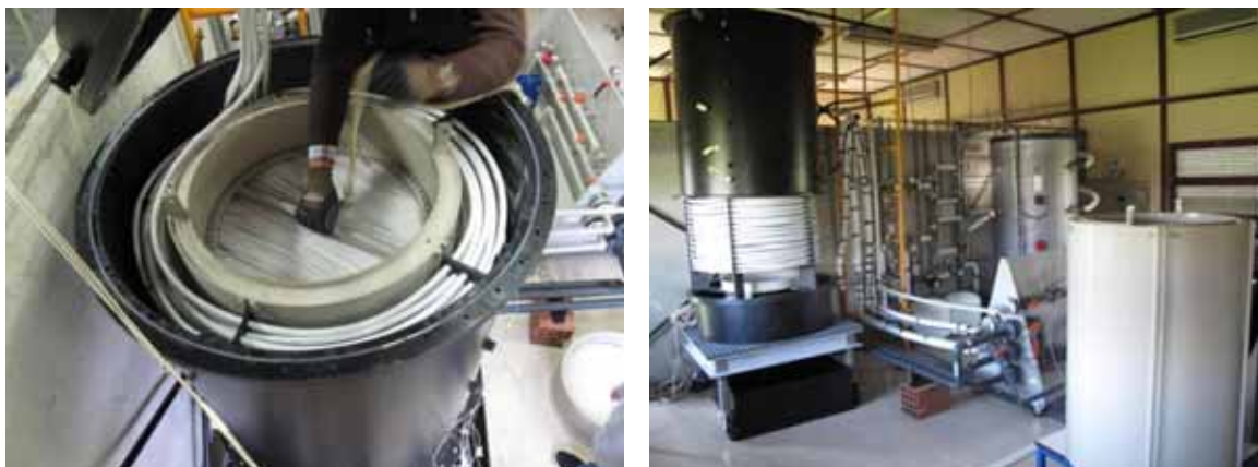
Fig. 3 – Assembled views of SELFWATER HDH prototype connected to the thermal test facility at LNEG laboratory. Left: stacked baskets with synthetic fabrics; Right: HDH prototype body with circular concentric chambers (condenser and evaporator).
