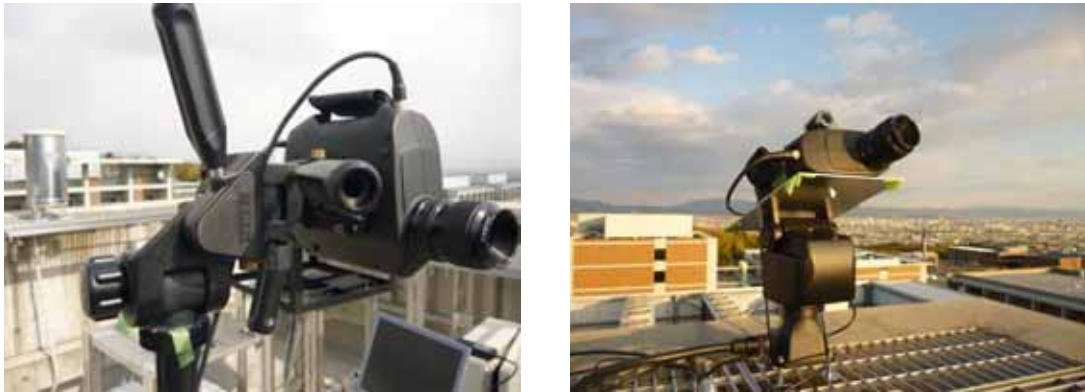
Fig. 6: Spectroradiometer on the angle scaled platform (a: left) and automatic pan-tilt unit controlled by a PC (b: right)
