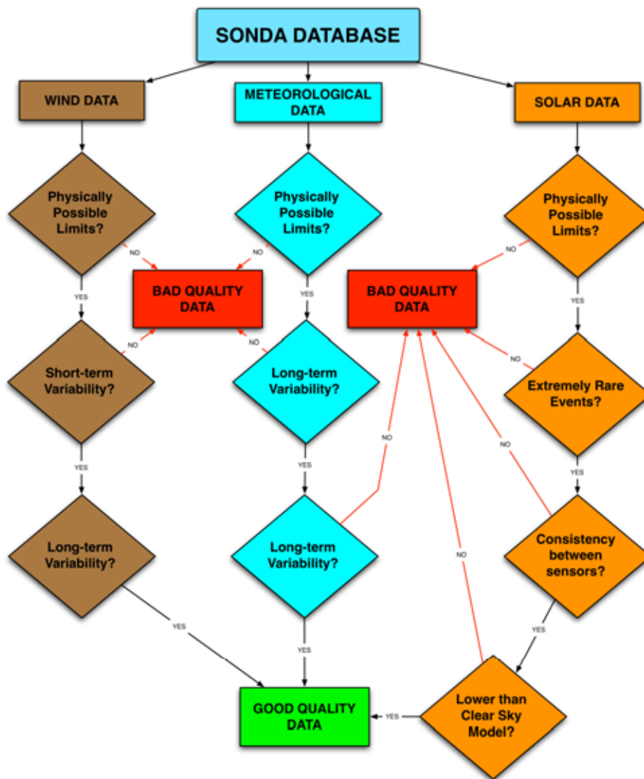
Fig. 3: Schematic Diagram for quality control algorithm used in SONDA database before deliver at INTERNET.
