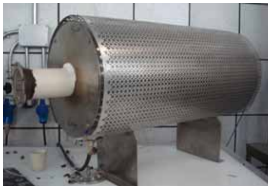
Figure 1: Tubular oven used for high temperature tests at CSIC-ICV
