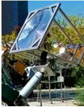
Figure 5: Pictures of the Fresnel lens used for thermal shock tests installed on solar tracker at CSIC-CENIM
