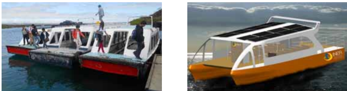
Fig. 1: Conventional ships operating in the Itabaca Channel (left) and solar powered catamaran designed to operate between Baltra and Santa Cruz islands (right).
