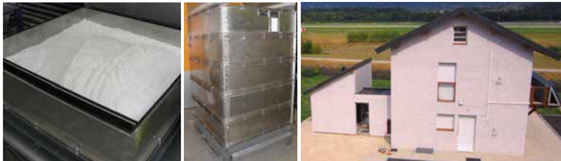
Fig. 6: Left to right : Salt fixed bed – 5 fixed beds assembled in one reactor – experimental house with its storage extension
