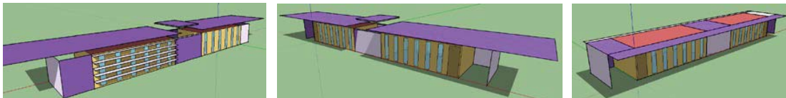
Fig. 3: Views of the office building (Model House) energy simulation done with SketchUp and Open Studio. From left to right: Solar protections, Cooling through natural ventilation, Thermal insulation in the roof.
