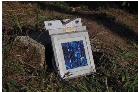
Fig. 6: R&S Renewable Energy Systems's irradiance measurer
