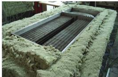
Fig. 6: Shell-and-tube LTES tank with fins.
