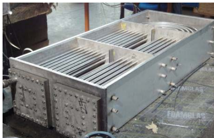
Fig. 5: Shell-and-tube LTES tank without fins.
