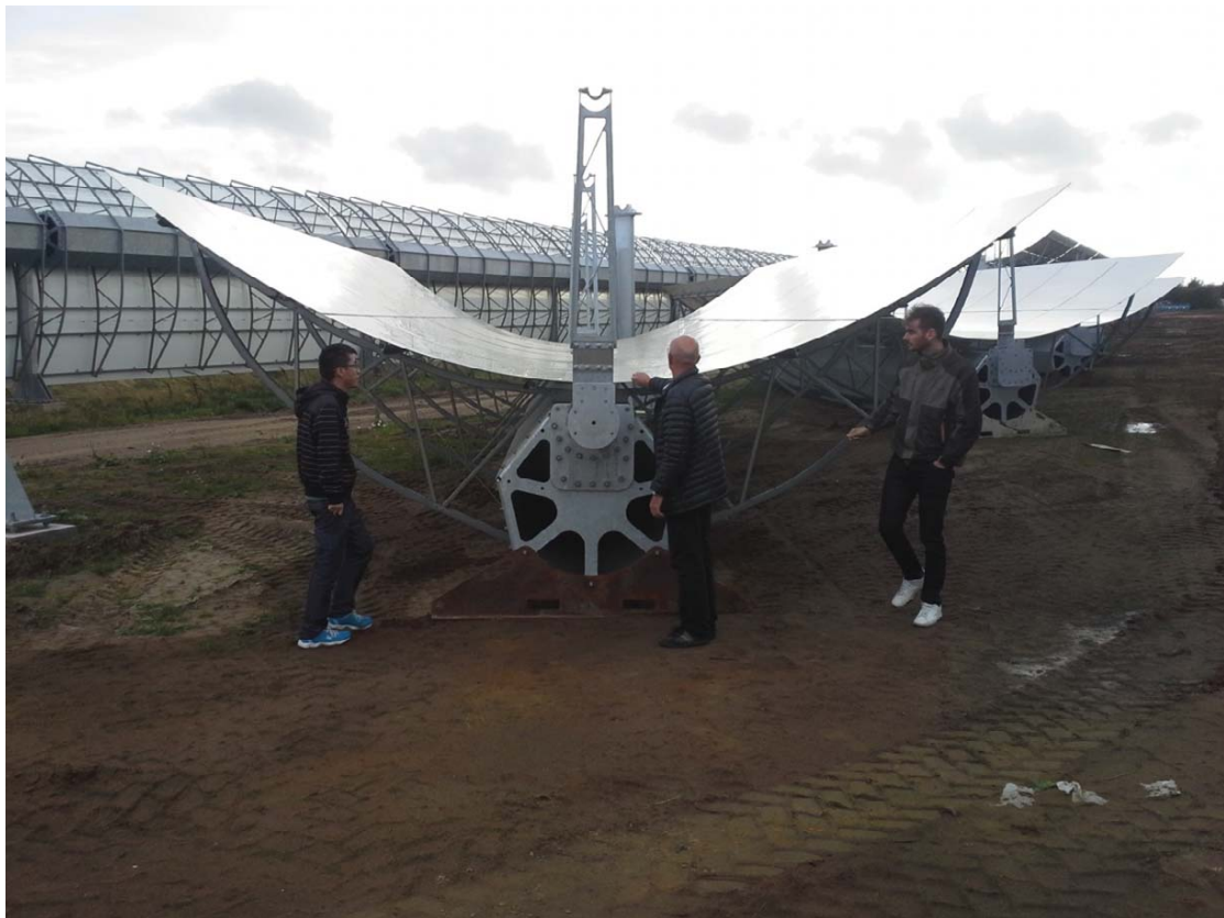
Fig 4. Close up of one mirror element of the CSP collectors. The width is almost 6 m. Glass mirrors are used. The metal structure is optimized for low material use, but till enough stiffness in windy conditions.
