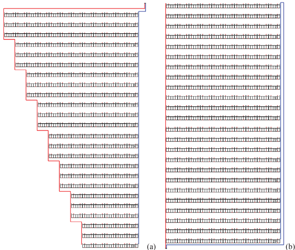
Fig. 6: Layout of the collector field assumed in case 2 (a) and in case 3 (b) (adapted from Arcon-Sunmark A/S).
