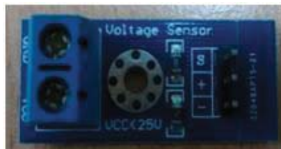
Fig. 5: Voltage sensor and connection diagram to arduino
