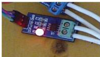
Fig. 6: Current sensor and connection diagram to arduino
