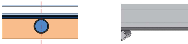
Fig. 2. (Left) Cross section of a pipe and its fin and (right) half a pipe modelled in COMSOL Multiphysics
