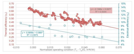
Figure 7 – Instantaneous thermal and electrical efficiencies
