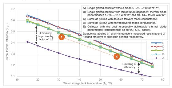
Figure 2 - Effect of diode thermal conductance upon diurnal thermal efficiency of an ICS collector
