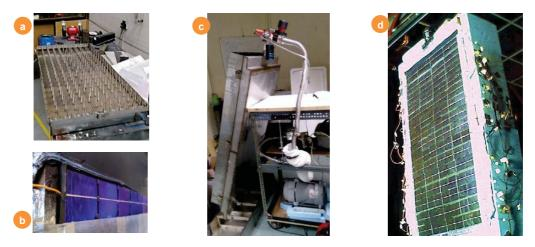
Figure 5 – Photographs showing steelwork & PVT absorber fabrication (a & b), leak testing (c), solar simulator testing (d)
