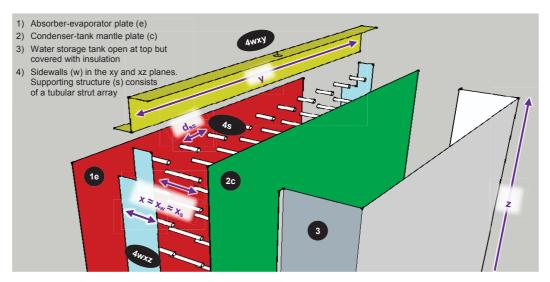
Figure 3 - Construction of the thermal diode and tank
