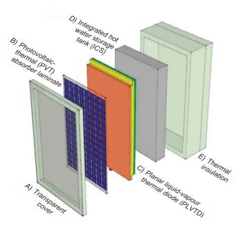
Figure 1 - General arrangement of a PVT-PLVTD-ICS solar collector
