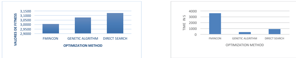
Fig. 14 Comparison of the different optimization methods: a) value of the fitness function b) time spent
