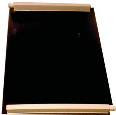
Fig. 4: Parallel flat-plate solar collector with rectangular manifold.
