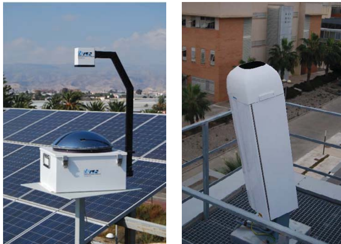
Fig. 1: Total sky camera, TSI-880 model and CL51 Vaisala ceilometer placed in the rooftop of the CIESOL building at the University of Almería
