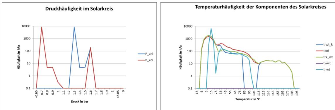
Fig. 4: Collector loop statistics of pressure and temperature in SHWwin
