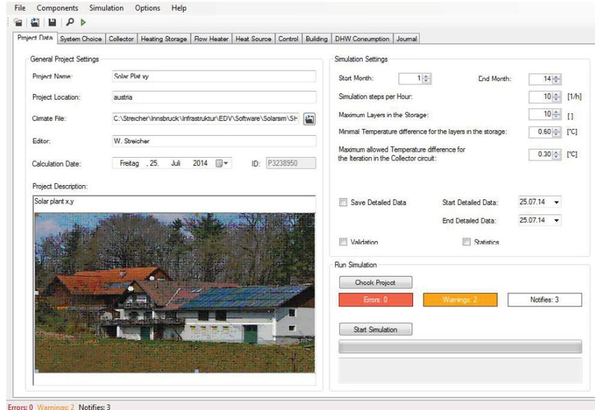
Fig. 5: System choice and visualization in SHWin
