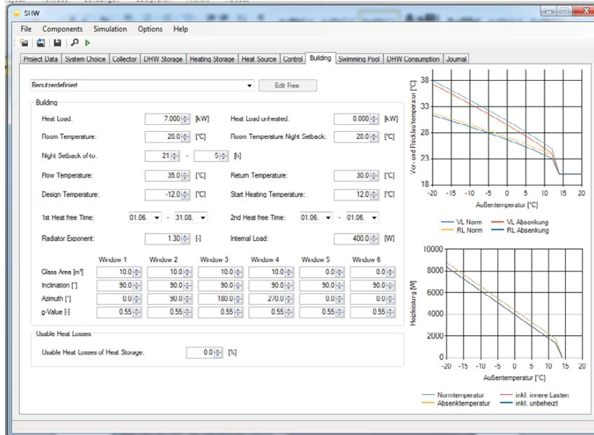
Fig. 10: Input and visualization of space heating demand in SHWin
