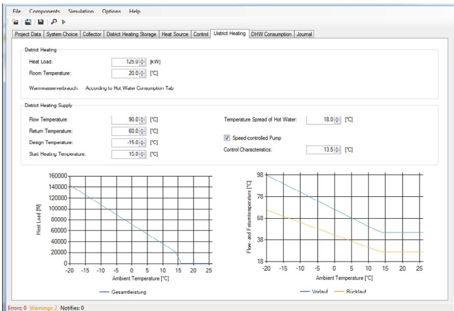
Fig. 11: Input and visualization of district heating network demand in SHWin
