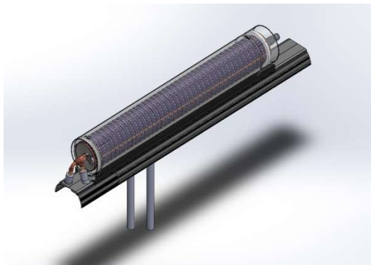
Fig. 8: Ridge profile, upper for the system, under profile to the beam of the ridge
