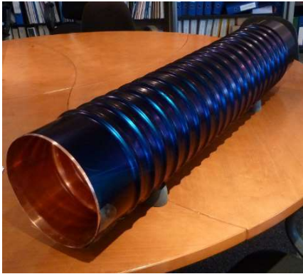
Fig. 6: Spectral layer on copper tube
