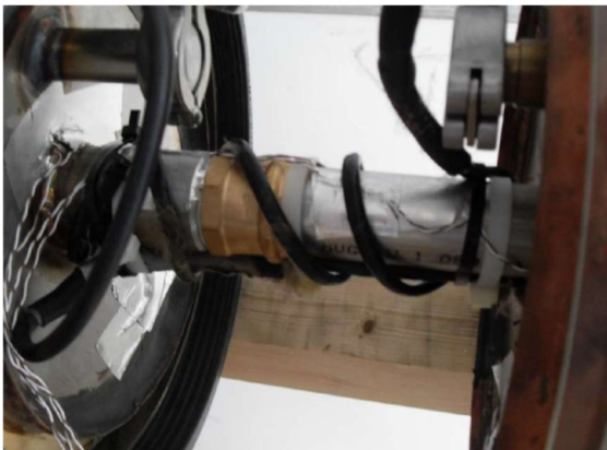
Fig. 13: Tracer on the connection pipe between the modules
