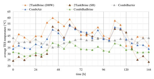
Figure 8: Average temperature of the TES-tanks during the 6-day system test.
