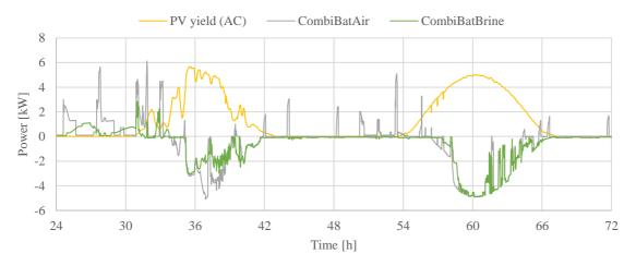
Figure 12: Excerpt of two system tests: PV yield (yellow) and the grid purchase (positive values green or grey) and feed-in (negative values) during a period of two days within the 6-day test.
