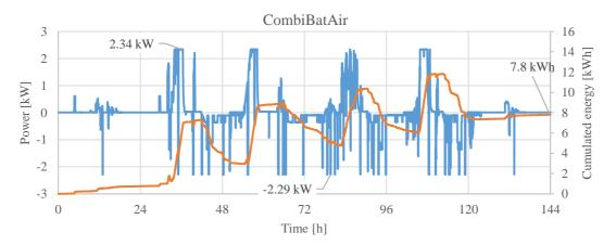
Figure 10: Electrical power of the charging and discharging of the battery as well as the cumulative energy during the 6-day test.
