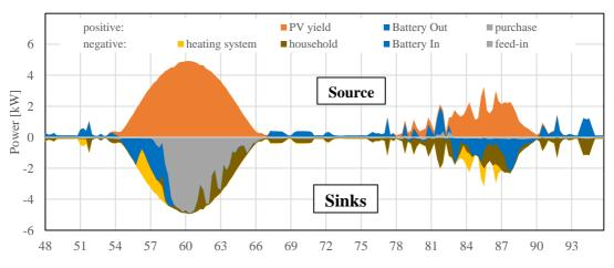
Figure 9: Excerpt of the measurement of System CombiBatBrine: Measurement of electric power during the days 3 and 4 of the 6day test sequence.
