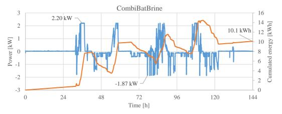
Figure 11: Electrical power of the charging and discharging of the battery as well as the cumulative energy during the 6-day test.
