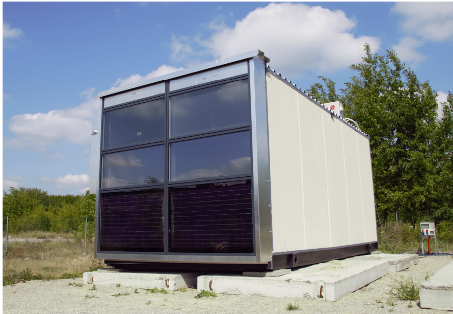
Fig. 4: Experimental test cell for energy-active façades
