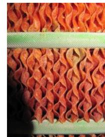
Fig. 3: Heat and mass exchanger design with corrugated wicking material
