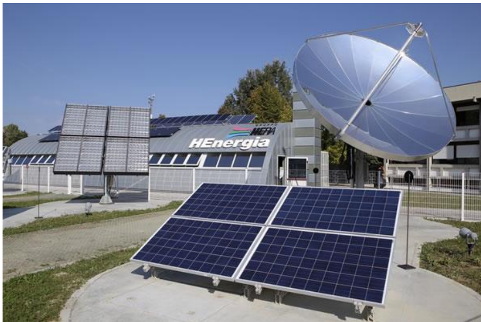
Fig. 2: Picture of the solar parabolic dish concentrator (on the right).
