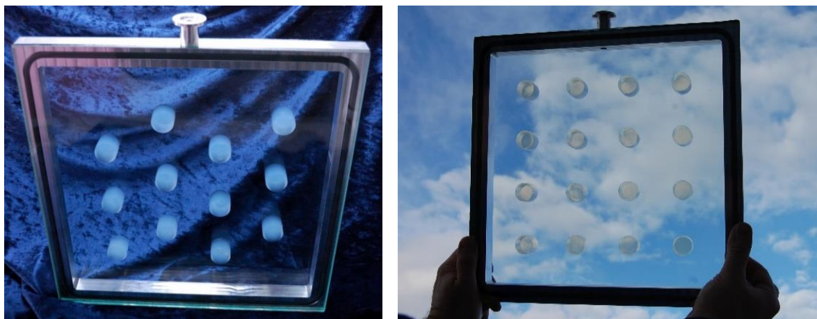
Figure 8: Demonstrators for evacuated double insulated glazing with silica aerogel pillars positioned in hexagonal (left) and cubic (right) arrangement.
