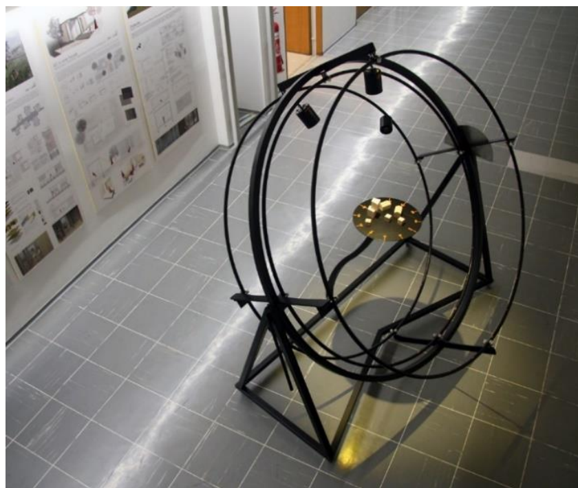
Fig. 1: Heliodon used for the educational purposes within the Bioclimatic design course held at UL FGG and UL ZF.
