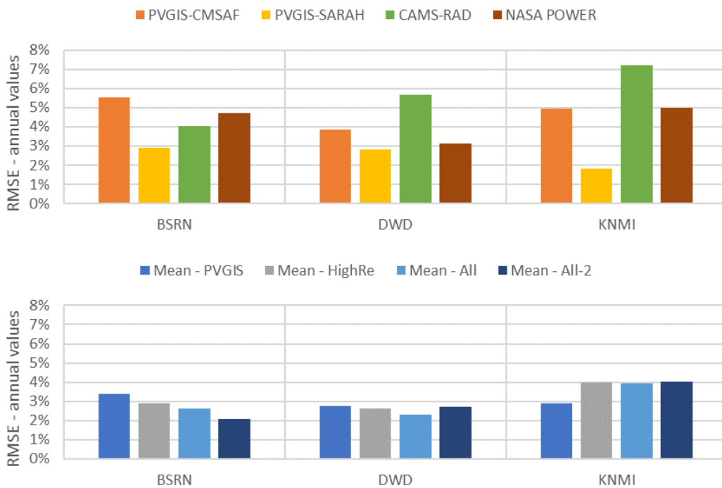
Fig. 2: Relative RMSE of annual values of different databases and arithmetic means as a function of reference sub-dataset
