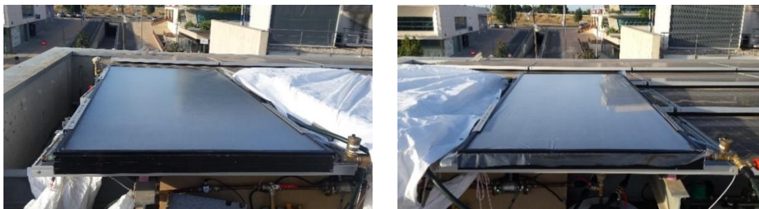
Fig. 1: Solar collector (left), and modified solar collector used as radiative cooling device (right).
