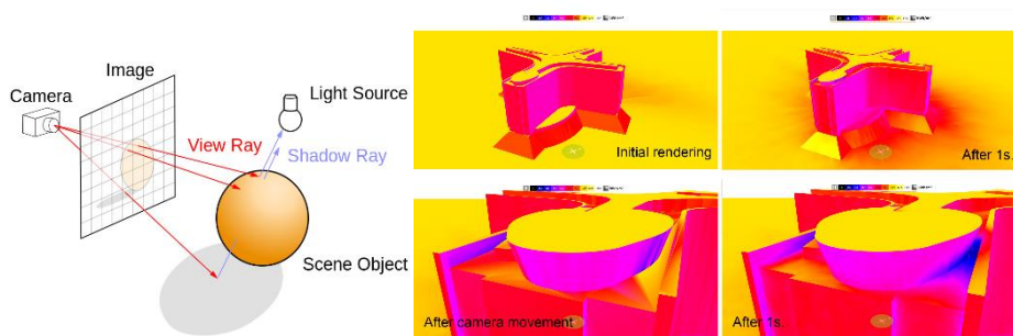
Figure 7: Raytracing principle – Irradiance rendering (sources: ©Wikipedia - ©ENERBIM)
