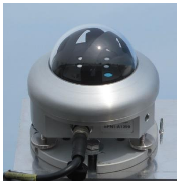
Figure 1: SPN1 sensor for the determination of diffuse and global irradiance
