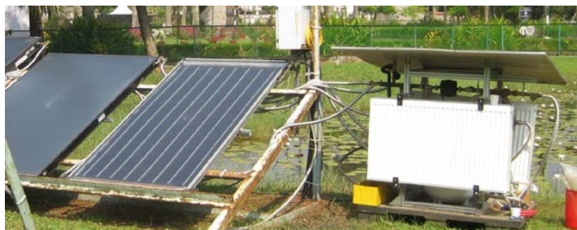
Fig. 2. Cooling unit (right) and collector 1 and collector 2 with combined temperature and humidity sensor (left) at the exposure site Kochi, India
