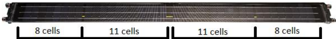
Figure 4: Receiver, showing 4 cell strings and its distribution in the receiver.
