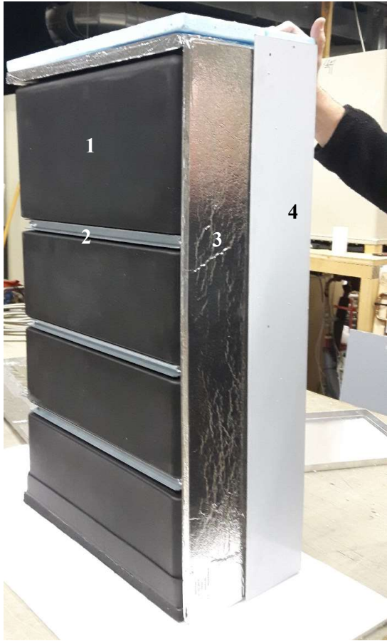
Figure 2: Photo of the storage tank vessel with metal reinforcement and VIP insulation.
