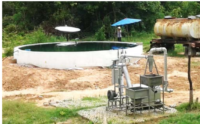
Fig. 8: Photos experiment fluidized – bed paddy dryer and solar pond
