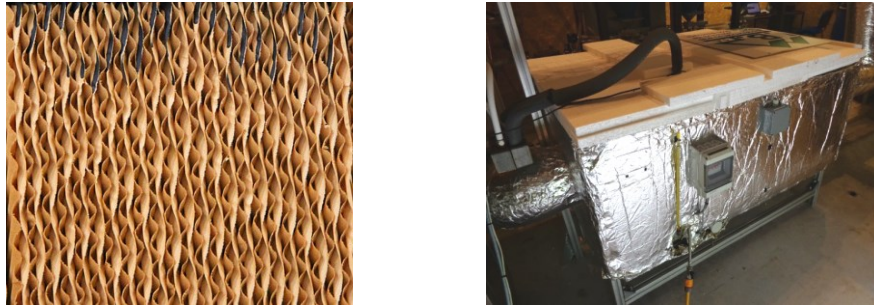
Figure 4 – (a) Evaporative cooling media; (b) Insulated box of wood integrating the evaporative panel. (D'Hondt, 2016).
