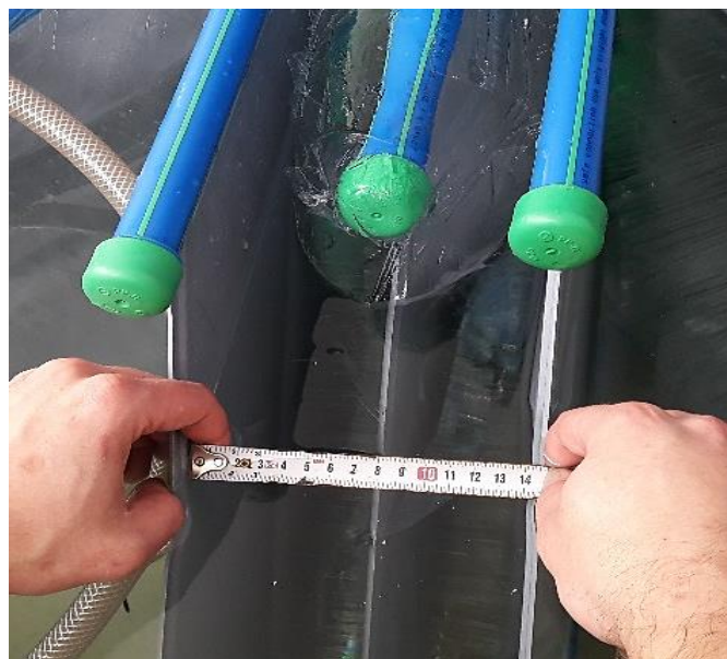
Fig. 10: Thickness of the ice walls of 14 cm from ice surface to ice surface with plate in the middle after one icing circuit with the star-shaped heat exchanger with 12 plates
