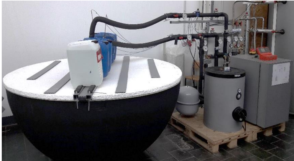
Fig. 1: Test bench with isolated ice storage (left), storage with heating rod (middle) and heat pump (right)
