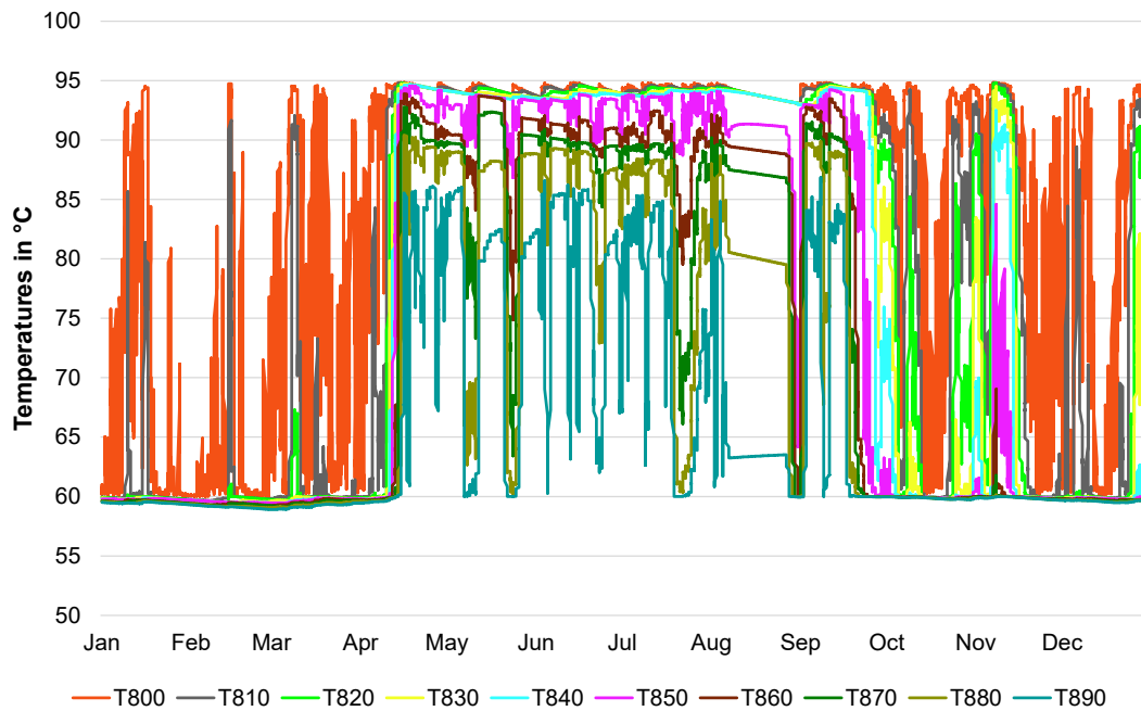
Figure 9: Temperatures inside the multifunctional heat storage over one year (TRNSYS simulation with 20 000 m 3 storage volume, waste heat profile 3)
