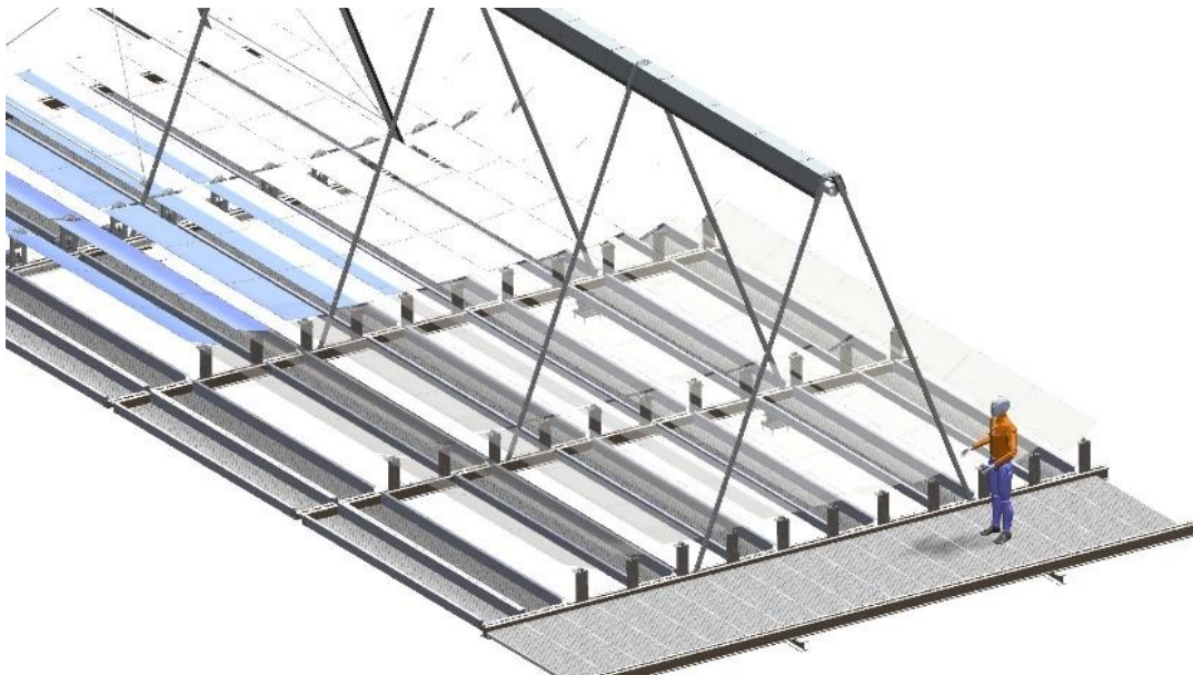
Figure 5 - Schematic configuration around a collector string
