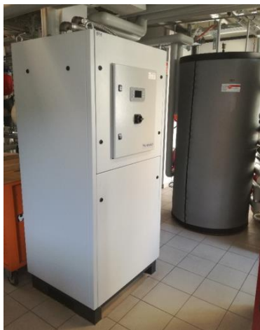
Fig. 4: Adsorption chiller Fahrenheit eCoo 10 and the emulated cooling load at the heat engineering laboratory
