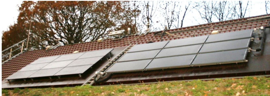
Fig. 2: Module test fields at the ISFH (left: PV module field; right: PVT field)
