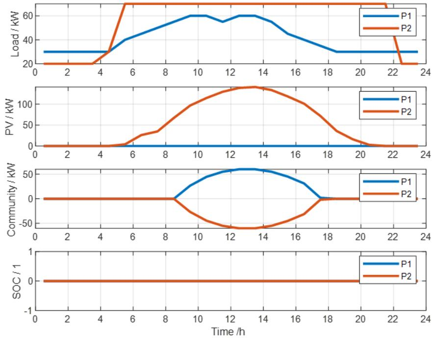
**Fig. 2:** First: Load profile of P1 and P2; Second: PV production; Third: Exchanged energy in the community, Fourth: State of Charge
