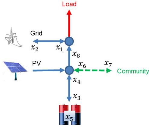
**Figure 1: Structure of energy flow optimization of one single participant in an energy community. States  $x_i$  consider power flow at every time instant**
