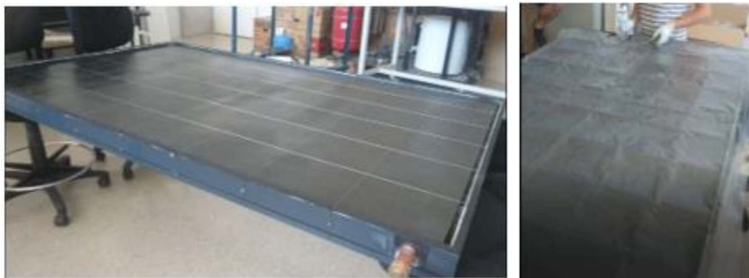
Figure 3: Nylon mesh located on the absorber in order to maintain straight the polyethylene film.
