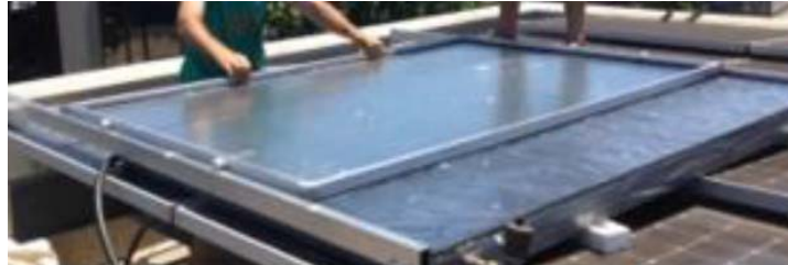
Figure 4: RCE device with the glass cover sliding over the aluminium guides.
