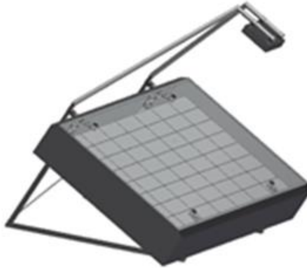
Fig. 1: Mirror-Box Concentrator with Receiver
