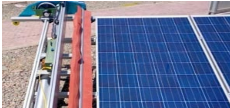
Fig.5: The Robotic Dust Mitigation (RDM) with silicon brush to clean the solar arrays [11]
