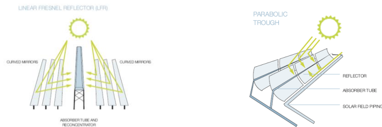
Figure 1: Linear focus CST technologies. Linear Fresnel collectors (left) and Parabolic trough collectors (right)
