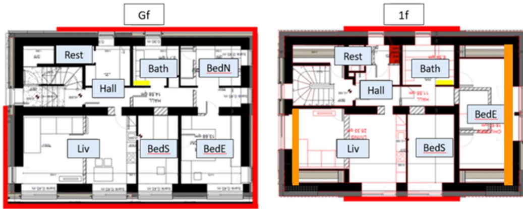
Fig. 5: Layout of the heating surfaces of the ground floor (Gf) and first floor (1f) of the building - ConExWall (red), electric radiator (yellow) and internal wall heating (orange).
