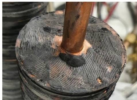
Figure 9 - sorbent ageing and peeling of the Copper fins: the sorbent shows an intrinsic ageing behavior after a 3 years exposure to sorbate vapor (left graph with the adsorbate loading in function of the age of the sorbent) and the sorbent disk peeled of the copper fin due to ageing of the glue (right picture).
