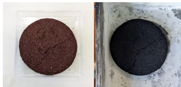
Figure 3 – SCG+RF monoliths before (left) and after (right) pyrolysis
