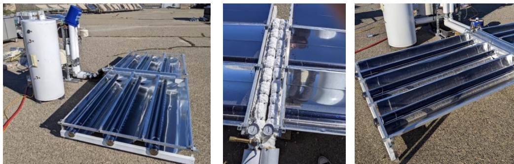
Figure 14. Prototype 1 and 2 undergoing long-term testing at temperatures >100 \text{ }^\circ\text{C}
