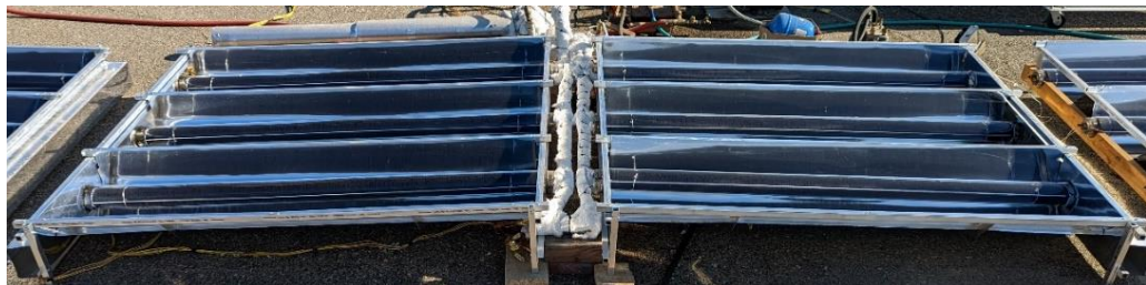
Figure 23. Gap losses and other optical losses due to reflector imperfections in NASH prototype modules.
